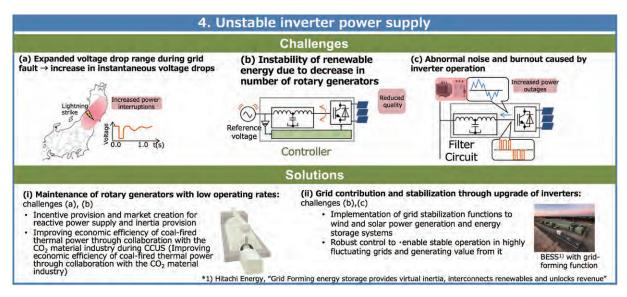
Figure 3.7 Issues and countermeasures accompanying large-scale deployment of inverter power supplies
