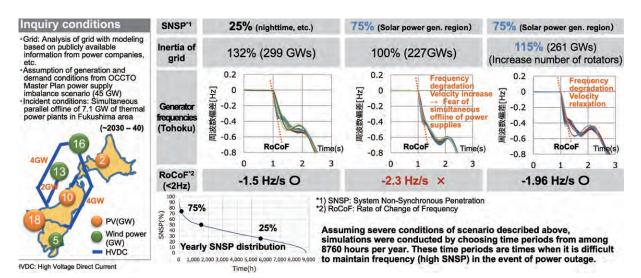
Figure 3.8 Frequency degradation due to drop in inertia and countermeasure by increasing the number of rotary generators
