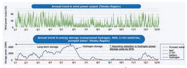
Figure 3.15 Example of annual transition in wind power generation and required energy storage<sup>36</sup>
