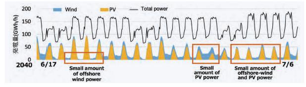
Figure 3.5 Example of a period with a small amount of solar/wind power generation ("use of nuclear power" scenario, Case 1', 6/17–7/6, 2040)
