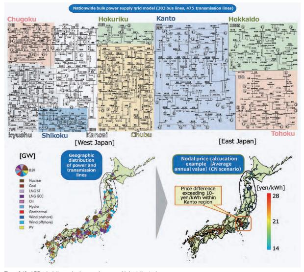
Figure 3.13 LDP calculations using large-scale power grid simulation tools
